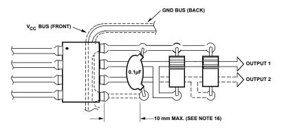
Figure 19. Recommended printed circuit board layout.
