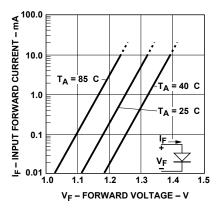
Figure 6. Typical diode input forward current characteristic.
