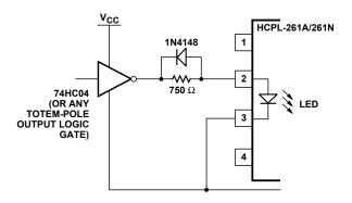
Figure 24. CMOS gate drive circuit for HCPL-261A/-261N families.
