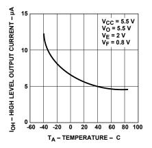
Figure 4. Typical high level output current vs. tem-
