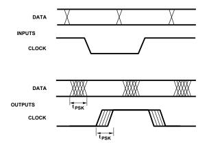
Figure 26. Parallel data transmission example.
