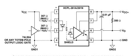
\*Higher CMR may be obtainable by connecting pins 1, 4 to input ground (Gnd1).
