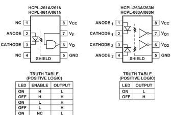
The connection of a 0.1  $\mu F$  bypass capacitor between pins 5 and 8 is required.
