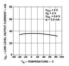
Figure 5. Low level output current vs. temperature.
