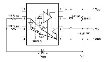
Figure 21. AC equivalent circuit for HCPL-261X.
