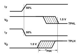
before the clock signal has arrived. From these considerations, the absolute minimum pulse width that can be sent through optocouplers in a parallel application is twice t<sub>psk</sub>. A cautious design should use a slightly longer pulse width to ensure that any additional uncertainty in the rest of the circuit does not cause a problem.
