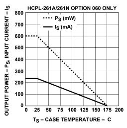
Figure 18. Thermal derating curve, dependence of safety limiting value with case temperature per IEC/EN/DIN EN 60747-5-2.
