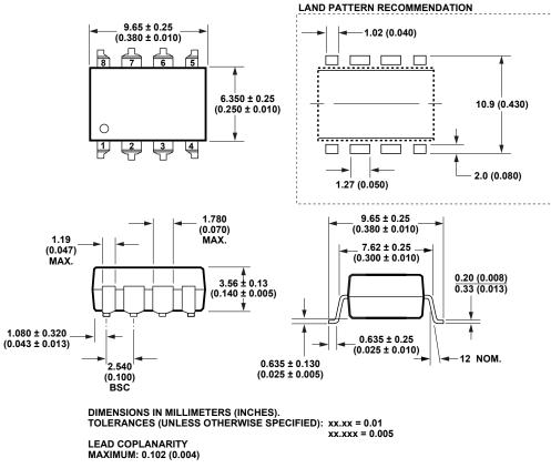
NOTE: FLOATING LEAD PROTRUSION IS 0.25 mm (10 mils) MAX.
