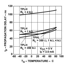
Figure 11. Typical propagation delay vs. temperature.
