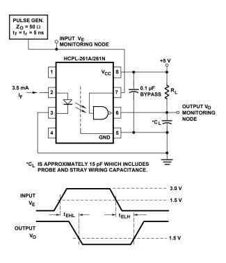
Figure 15. Test circuit for t<sub>EHL</sub> and t<sub>ELH</sub>.
